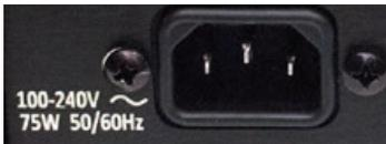
Plug the power cord that comes with your amplifier into the AC inlet on the rear. Any 3-prong IEC cord may also be used with the amplifier. Always ensure that the ground contact is intact on both the cord and receptacle.
