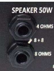
Connect a single 8 or 16-ohm speaker to the lower jack, 8-OHMS.
