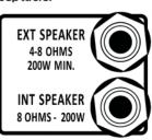
connecting the external speaker. An external 4 ohm speaker cabinet should be connected to the upper 4-8 ohm **EXT SPEAKER** output.
