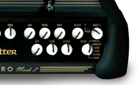
Turning up the overdrive limiter (LIM) progressively reduces master overdrive distortion (but not Cream or Crush), while maintaining lower-level sustain, effectively replacing the "brick wall" of overdrive distortion with a "soft cushion" of limiting.
